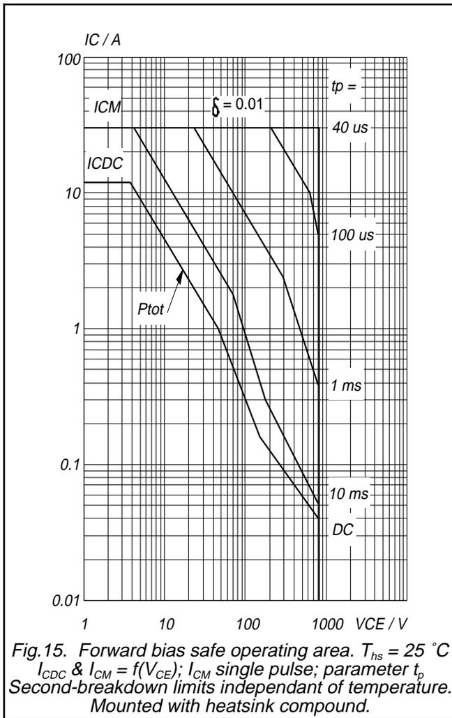
Fig.15. Forward bias safe operating area.  $T_{hs} = 25\text{ }^\circ\text{C}$
