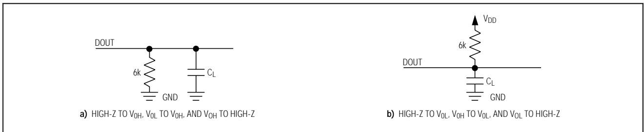
Figure 1. Load Circuits for Enable and Disable Time
